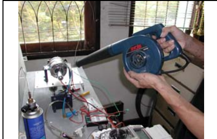
Bench start and blower for added safety and extra cooling
